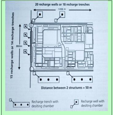
Figure 5.1: Diagram of Typical Sector for Recharge Wells
